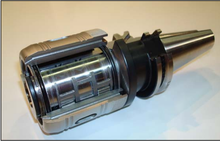
Fig. 3.19 Section of a “great power” collet chuck, by Laip ® , showing the internal needles to make the radial force
