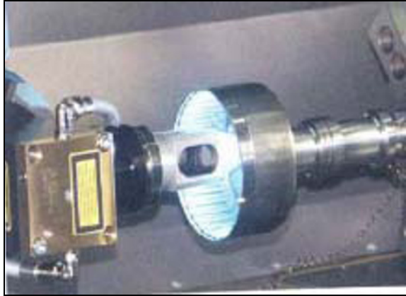
Fig. 7.15 Laser welding integrated in a turning centre, by Boehringer®
