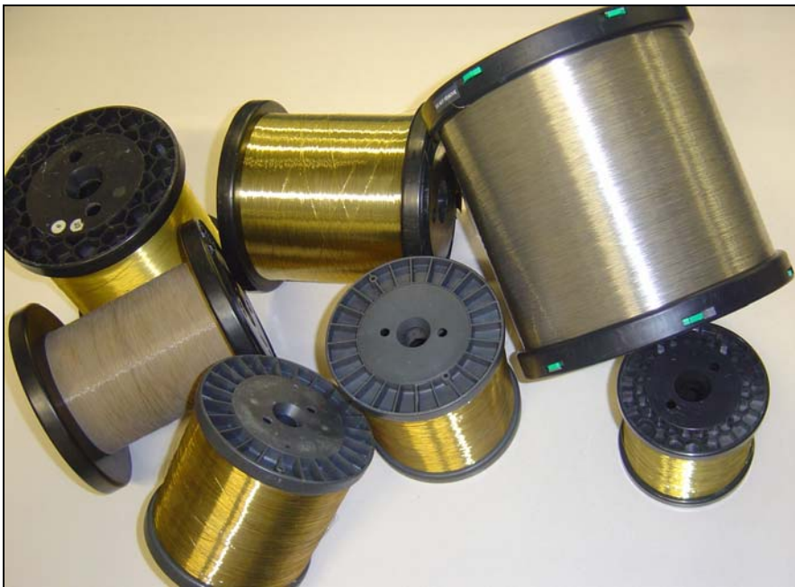
Fig. 9.15 Wires for WEDM
