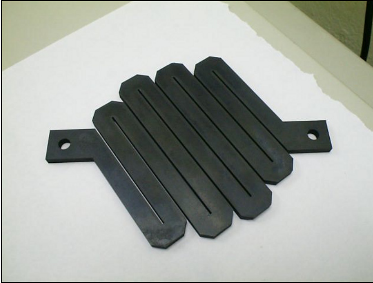
Fig. 9.16 Heat exchanger cut by WEDM. The material component is silicon infiltrated silicon carbide
