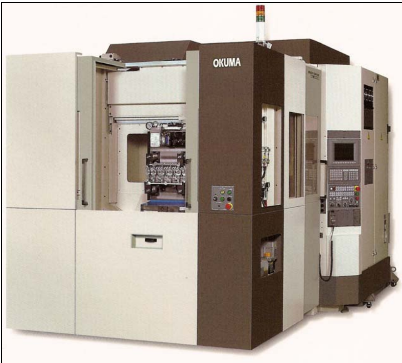
Fig. 13.9 Example of a 4-axis high performance machining centre, by Okuma®
