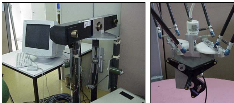
Fig. 10.12 Calibration of a 4-DOF PKM robot [2], the camera and target
