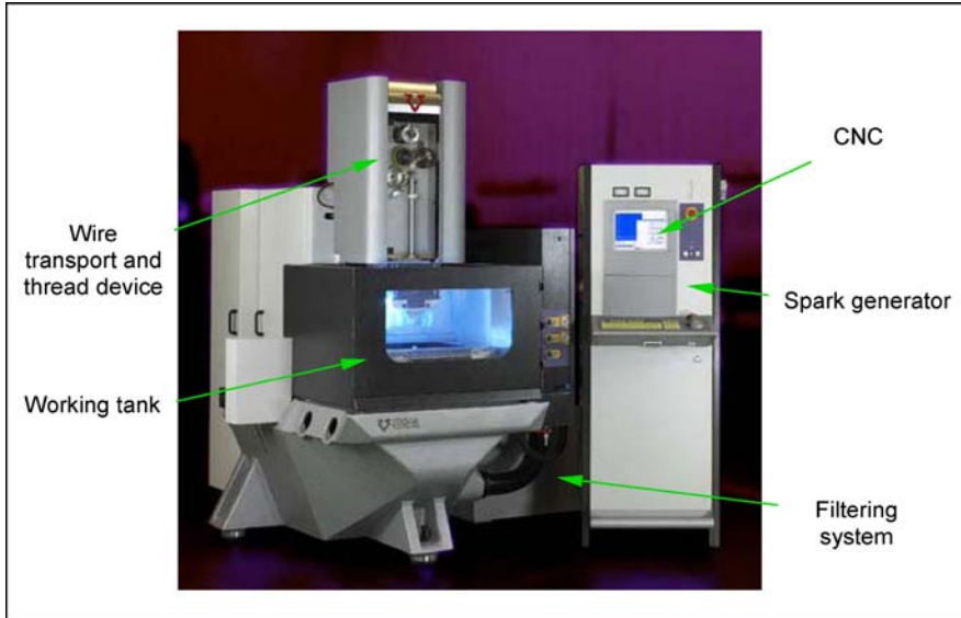
Fig. 9.10 Main systems of a WEDM machine. The photograph shows an ONA ® AX300 wire EDM machine [21]
