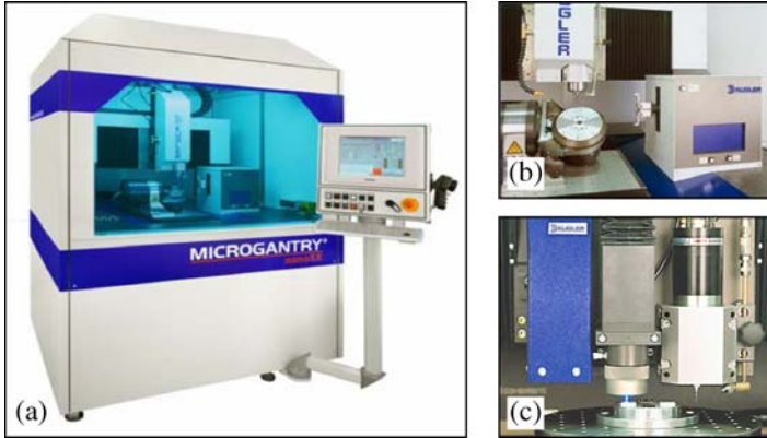
Fig. 11.26 Kugler ® Microgantry nano 3/5X. a A general view. b Rotational CNC axes. c Laser and milling heads
