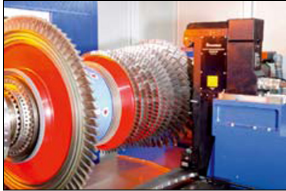
Fig. 8.20 Laser measurement in tip grinding of turbine blades, by Danobat®
