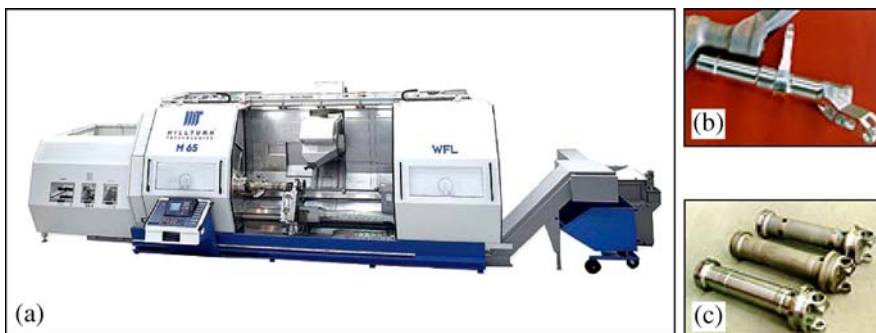
Fig. 12.18 a Millturn 65 from WFL® and some examples of manufactured parts. b Flap lever. c Landing gear
