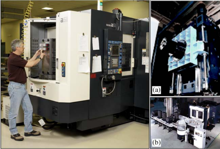
Fig. 1.23 Horizontal machining centre, model Makino® a51. a Detail of the spindle and column of Makino's A77. b Automated system for production of engine blocks
