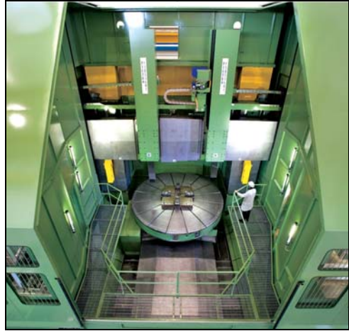
Fig. 7.8 Heavy-duty vertical turning centre, AC 46 by Pietro Carnaghi®
