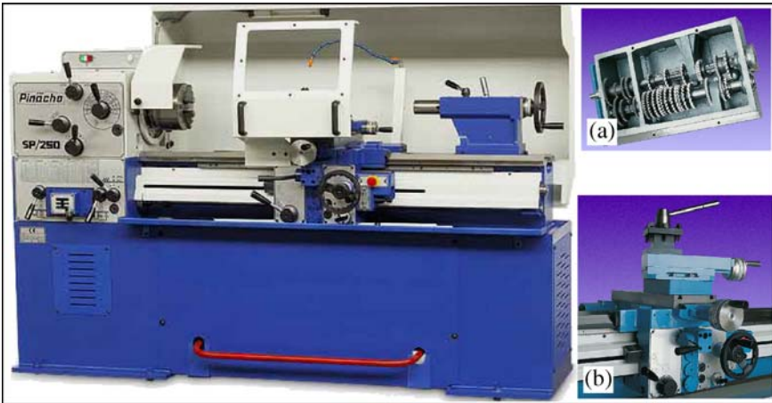
Fig. 1.28 Engine lathe, model SP250 by Pinacho®. a Detail of the feed gearbox. b Universal turret
