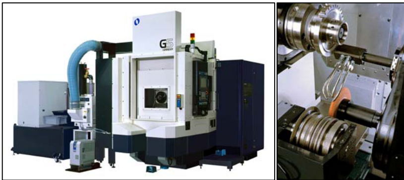
Fig. 12.15 Horizontal machining centre G5 iGrinder from Makino®
