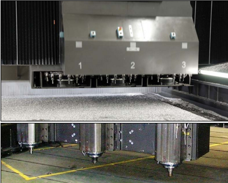
Fig. 3.7 Two images of the Nicolas Correa ® Neptune, an example of multi-spindle configuration
