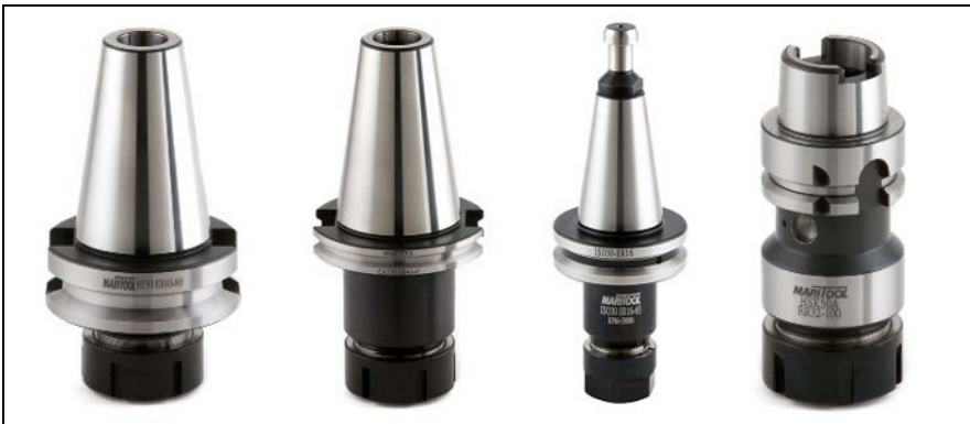
Fig. 3.16 Standard toolholders by Maritool ® , from left to right: BT50, CAT50, ISO30, HSK50A
