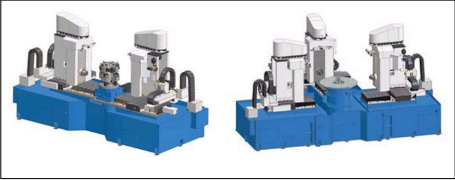
Fig. 13.7 Modular rotary transfer machine with automatic tool changer per station, by Ultra Tech Machinery®
