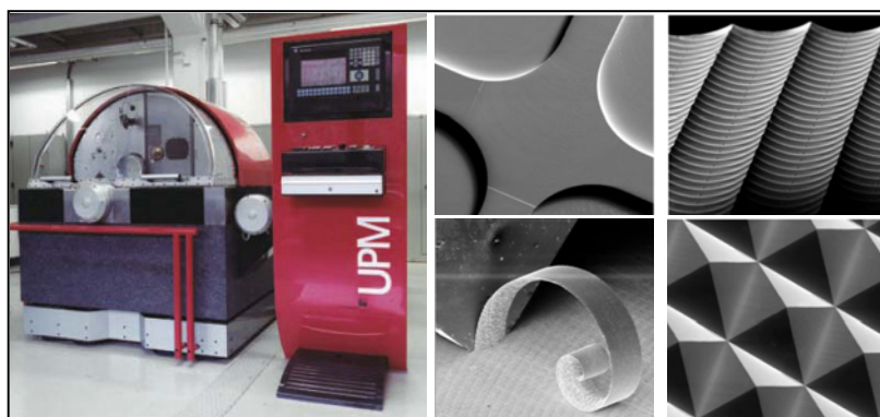
Fig. 11.5 3 axis ultraprecision milling machine with diamond tools and some application cases (courtesy of Fraunhofer IPT)
