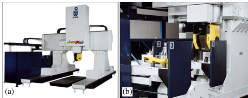
Fig. 12.19 a JomaX 265 from Jobs ® . b Automatically interchangeable spindles
