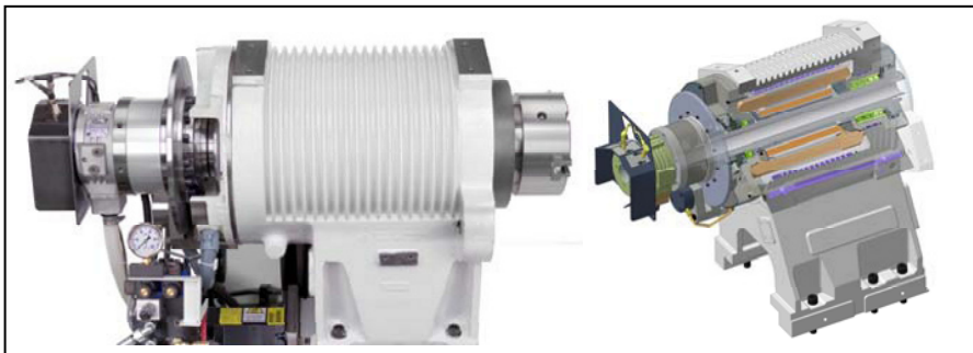
Fig. 6.5 Total design principle: built-in motor embedded in a lathe spindle, by CMZ Machinery Group ® . The spindle is refrigerated with oil
