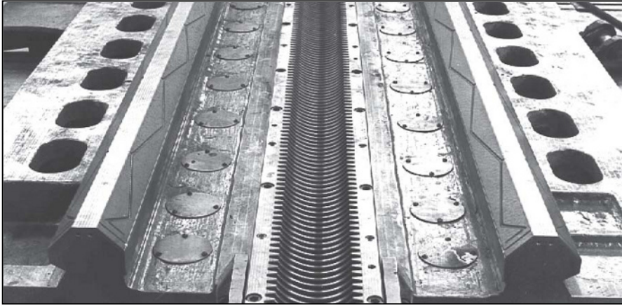
Fig. 4.19 Coated slideways and worm rack in a table of a gantry milling machine (by SKC ® )
