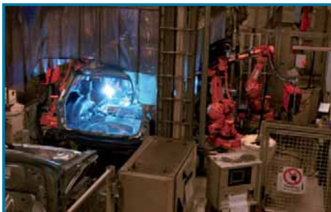
Fig. 7. The CMT system enables Volvo to reduce cycle times in the pressing plant.
