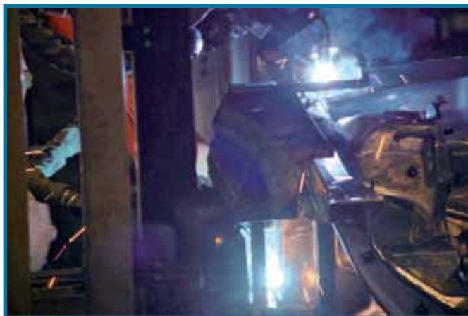
Fig. 5. The CMT systems join high-strength hot-stamped steels such as Boron and Usibor to the body shell of the Volvo “V 70” with almost no spatter.
