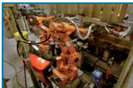
Fig. 3. The CMT systems have been integrated into the production process and the existing welding cells without having to modify the body shells.
