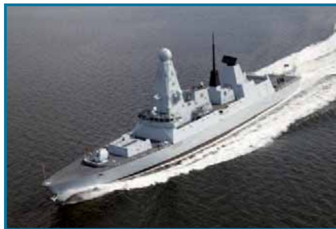
Fig. 1. A Type 45 destroyer with a top side containing a significant proportion of 4 and 5 mm thick plate.
