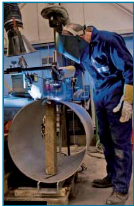
Fig. 2. High temperature proven during formation, the processed expanded silicate "Rotocell" plays a critical role during the submerged arc welding process with its important contribution to quality and efficiency.
