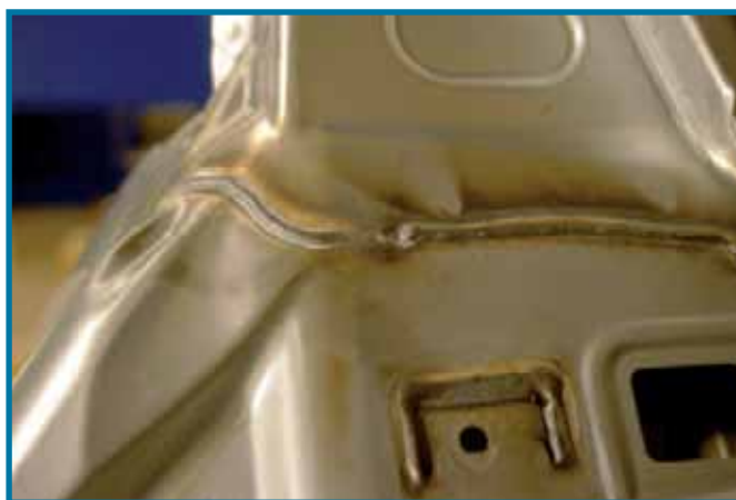
Fig. 2. Four seams join 1 mm thick sheets in the body shell area between the wind-screen, A-pillar and the front side panel.
