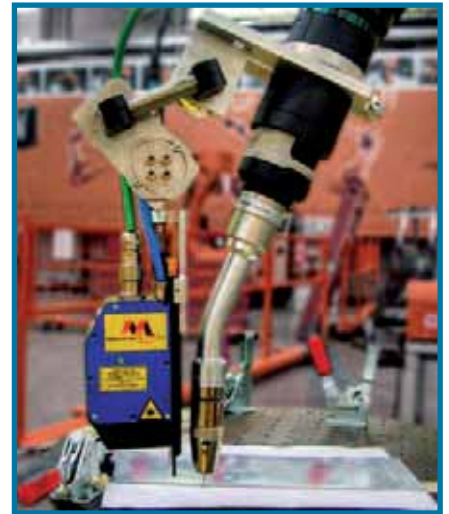
Meta's new "Smart Laser Pilot" laser-based seam tracking system for robotic welding.
