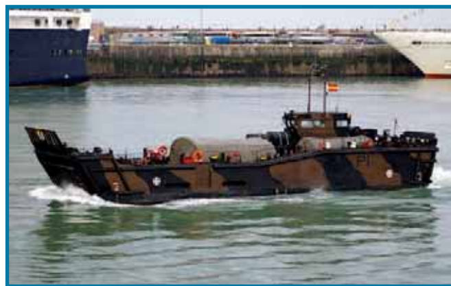
Fig. 2. A Landing Craft Unit (LCU) which contains significant quantities of 4 mm thick plate.
