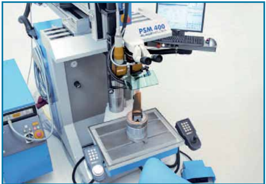
Fig. 1. The “Blade Welder” is suitable for machining turbine blades and high-alloyed tool steels.
