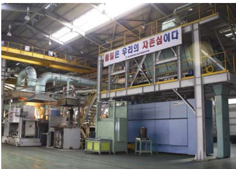
In addition to the DISA 240-C moulding line, DISA also supplied the complete sand plant and pouring furnace solution
