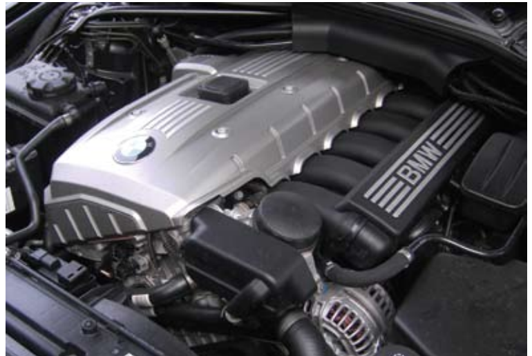
BMW three litre engine block using lightweight magnesium
