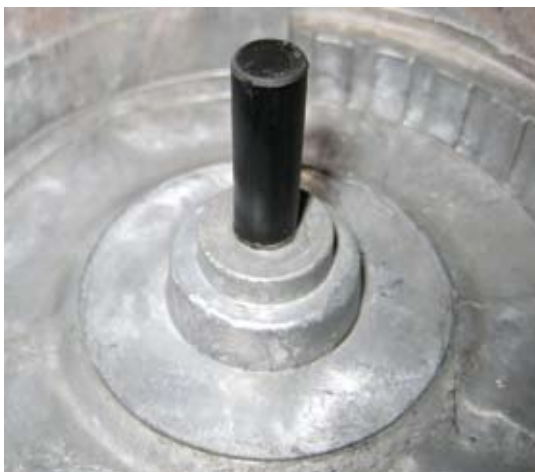
Fig 2. Test bar embedded into a pressure diecast part
