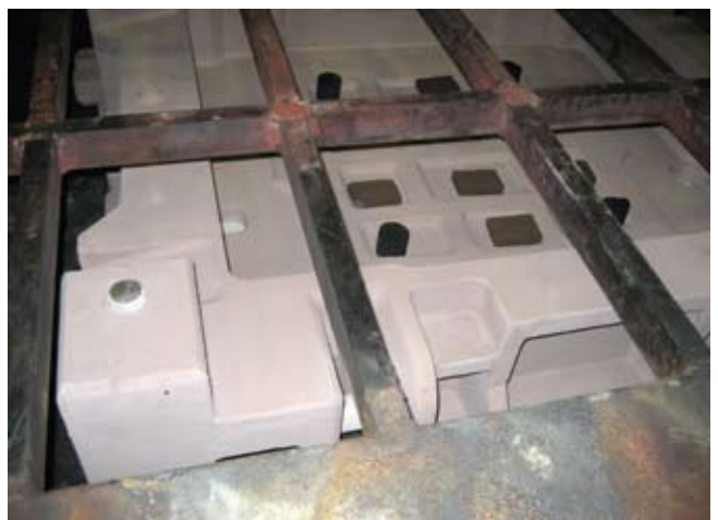
Ready to cast using the lost foam method in the existing foundry
