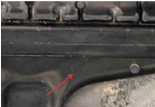
Fig 2. Test core after 55,964 shots. The core is in very good condition, without any visible heat cracks although the bore shows initial heat cracks
