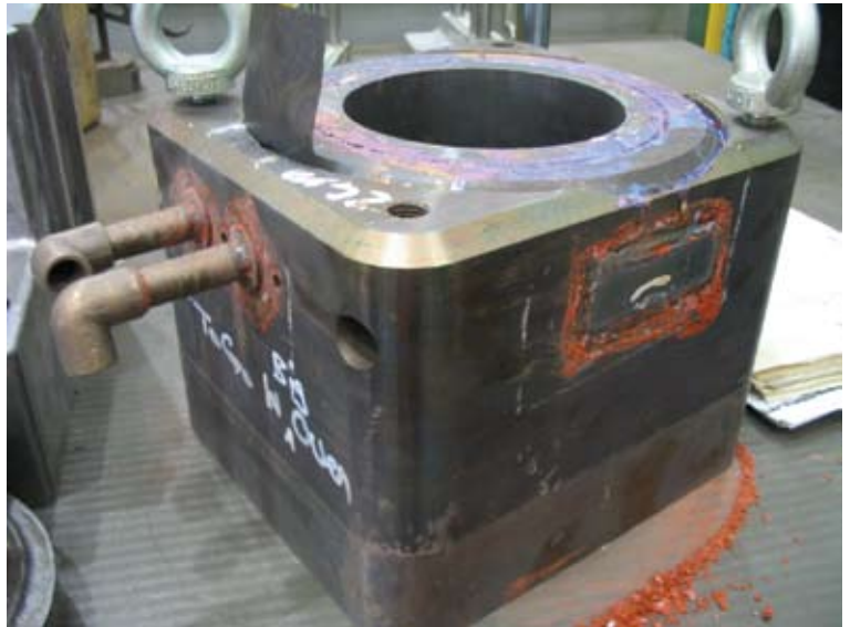
CASTrepair successfully applied to a leaking sprue bush due to cracks. The two sleeve inserts shown are cast in with CASTrepair alloy
