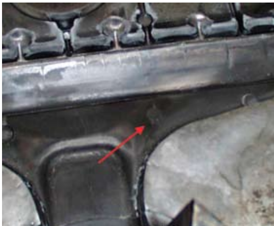
Fig 3. Test core after 71,282 shots. The core is in very good condition, there are no visible heat cracks although the bore shows increased heat cracks
