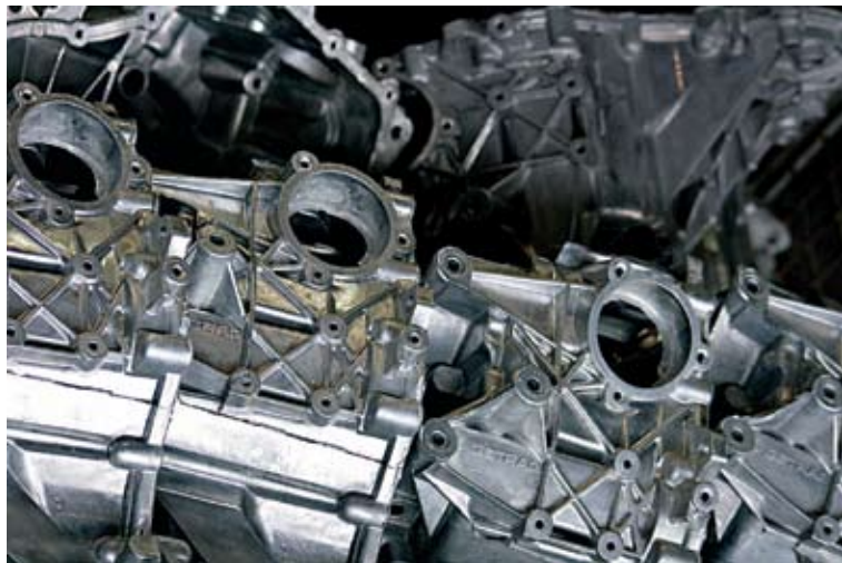
Engine blocks cast at Nemak are made with a 25% faster cycle time using robots
