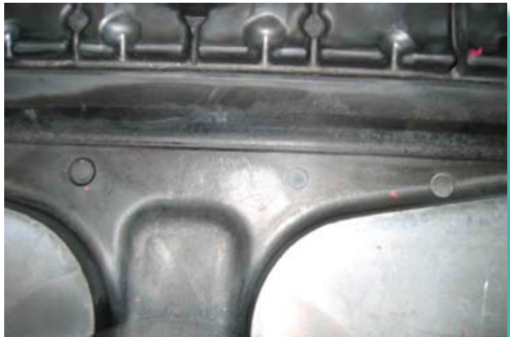
Fig 1. Test core after 104 shots: the core has the same characteristics as a normal core, no cracks or irregularities being visible
