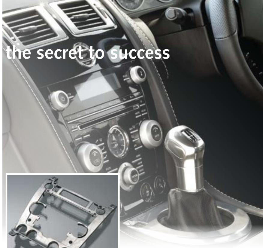
Centre console for Aston Martin, produced as a high pressure diecasting; prepared and ready for paint or veneer
