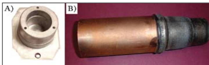
Fig.12 (a) casting; (b) H13 laser-deposited over copper core
