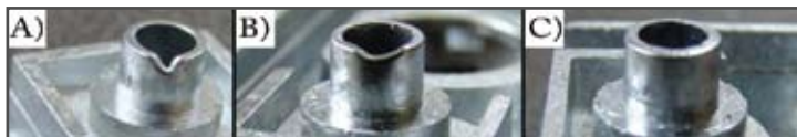
Fig.11 This casting had fill issues, but the new alloy eliminated scrap due to lack of fill
