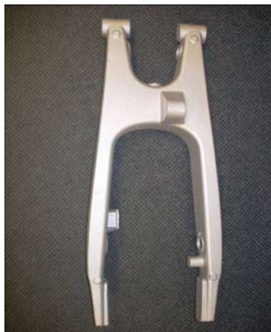
Fig. 9 An aluminium alloy B206 (Al-4.5Cu) alloy swing arm casting, 2.5 mm thick wall, with isolated unfed bosses, notably free from hot tearing, characteristic of this alloy
