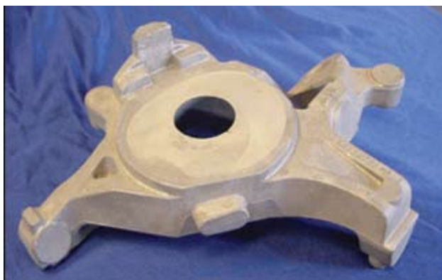
Fig. 8 Example of casting in production using ablation casting process, knuckle component
