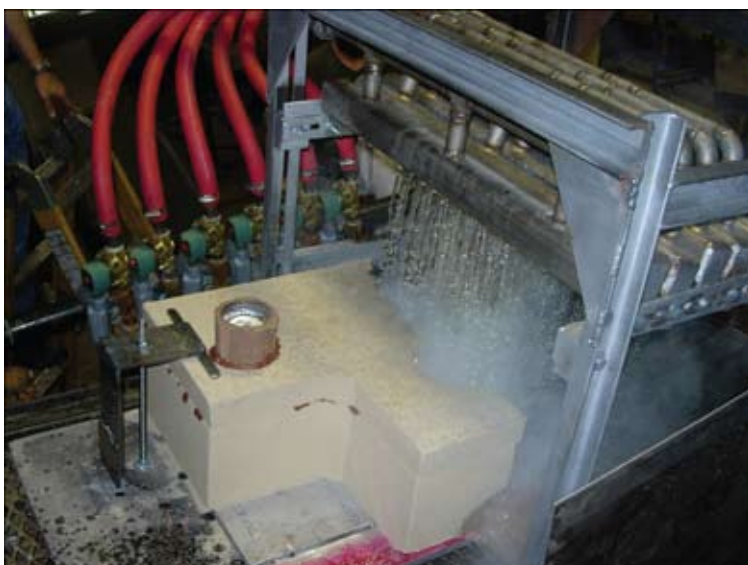
Fig. 1 The ablation of the mould in progress
