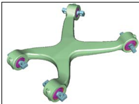
Fig. 3. The forged X-link assembly
